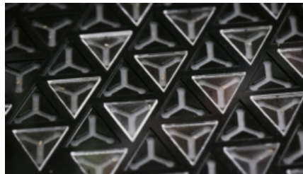
This array of Y-mazes is used to track fruit fly behavior.
